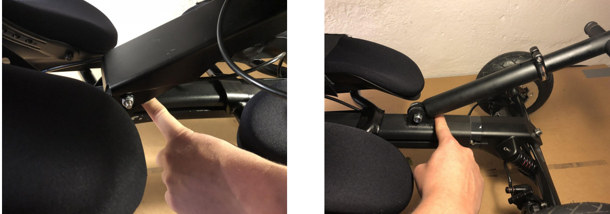
Figure 6.4.1 - Danger of trapping fingers during folding.
