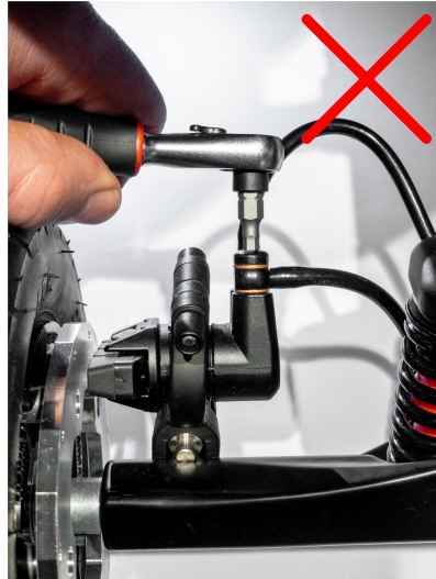
Figure 6.3 - NOTE! Do not adjust this screw. Adjustment of this screw may lead to leakage
