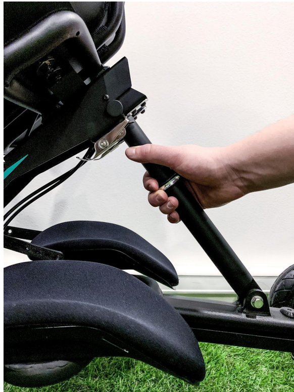
Figure 3.4.5 - Risk of trapping fingers
