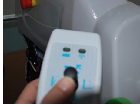
Fig. 70 Press any command to calibrate the maximum operating distance.
