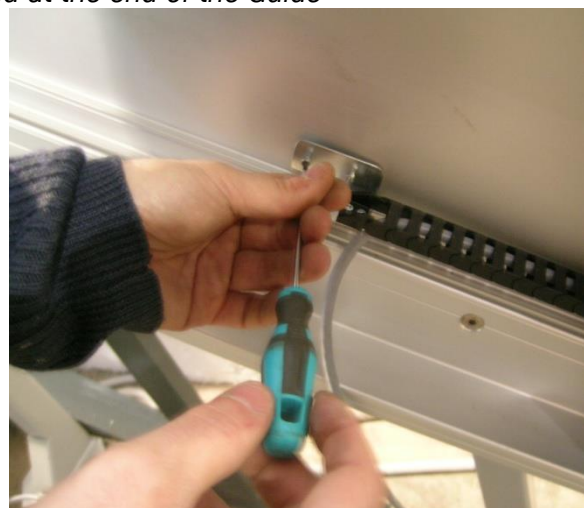
Fig. 20 – Detail of fastening chain to the guide
