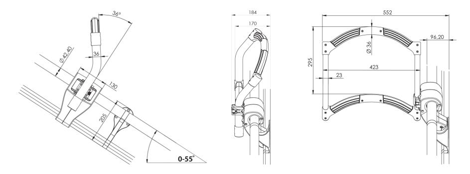
Measurements are in millimeters and degrees. All dimensions measured from the wall is nominal and may change, depending on required installation accessories required in each individual case. Maximum user weight is 120 kg / 264 pounds. \*Additional accessories on top of base configuration might be required. \*Compatible with outdoor conditions where snow and ice cannot reach the railing system.
