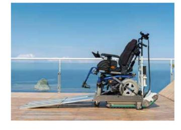
Secure the wheelchair using the supplied straps and store the telescopic ramps in the appropriate housings.
