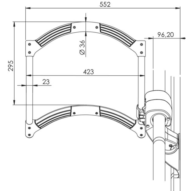
Measurements are in millimeters and degrees. All dimensions measured from the wall is nominal and may change, depending on required installation accessories required in each individual case. Maximum user weight is 120 kg / 264 pounds.
