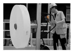
Lifting trolleys offer easy and ergonomic lifting, moving and tilting of goods such as rolls and drums, with full flexibility and mobility.
