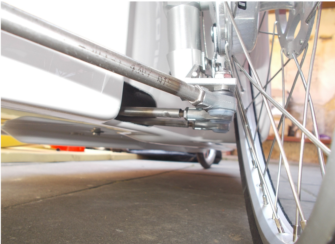
Improved steering geometry for better stability, new precise fitting bearings.
