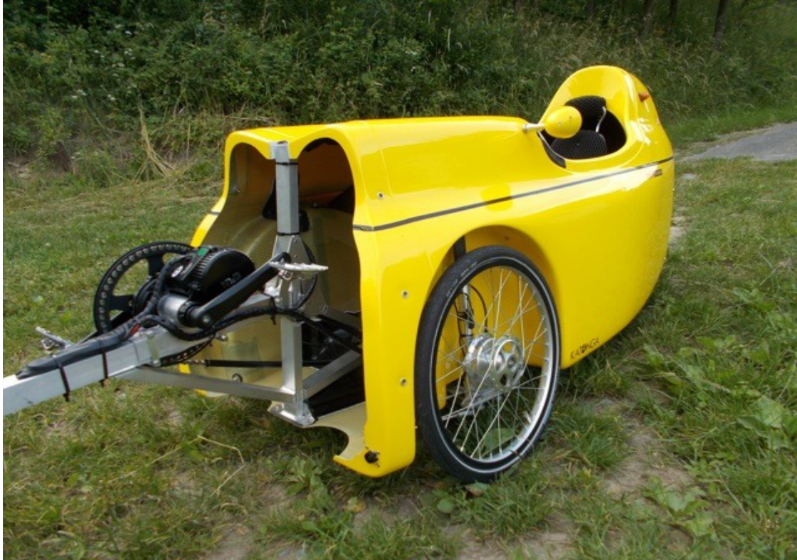
WAW256 velomobile equipped with Bafang Electric assist. 250W /25 km/h, Lithium ION 24V - 15 Ah battery
