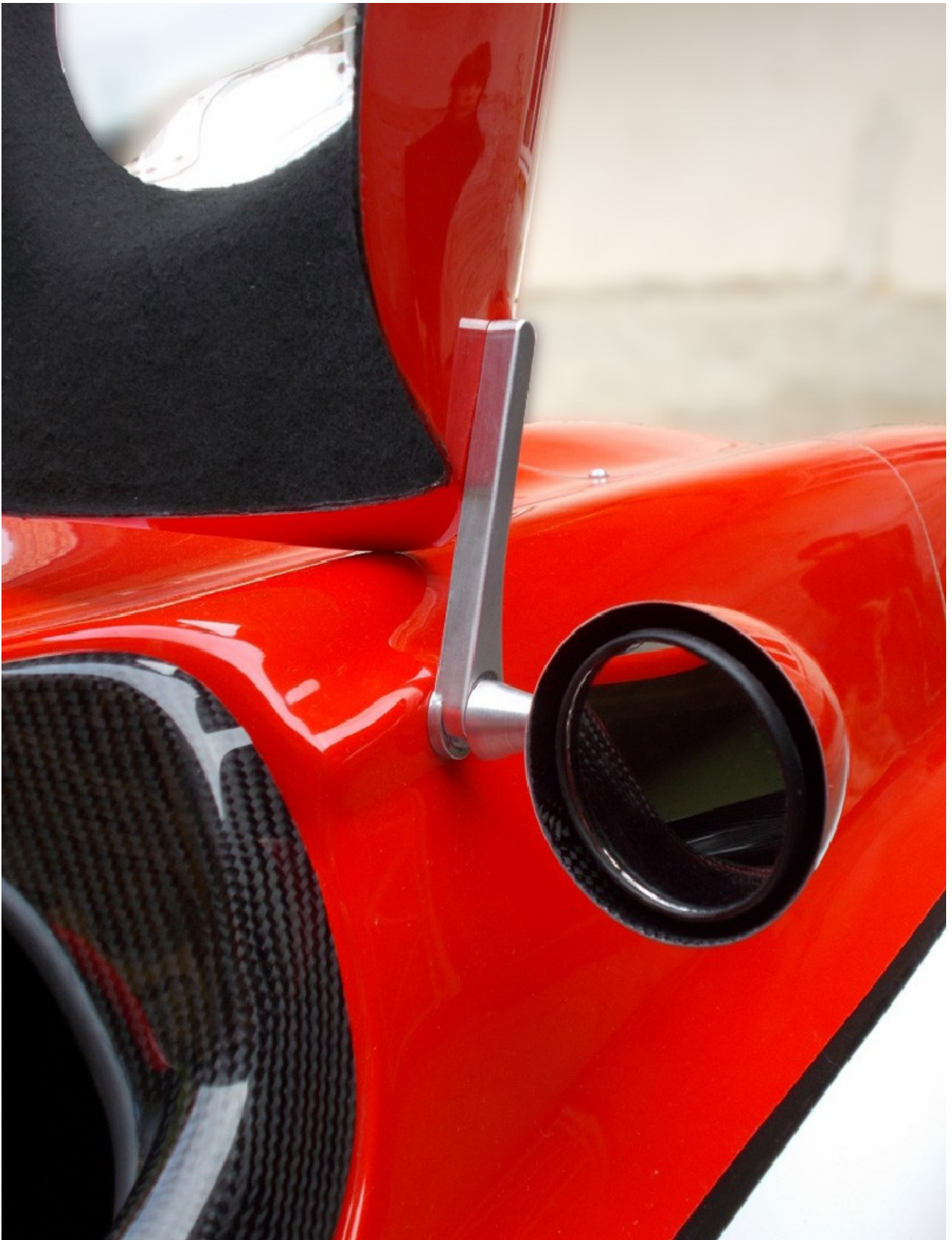
Racing hood attachment and aerodynamic mirrors. Acoustic felt for sound damping.
