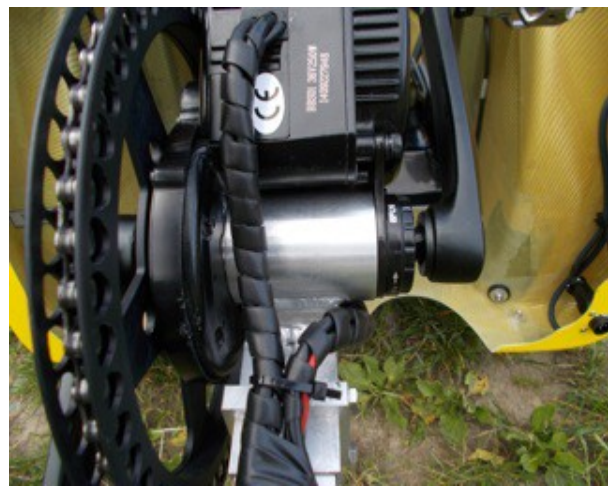
Trouseguards outside chain wheel (50t).
