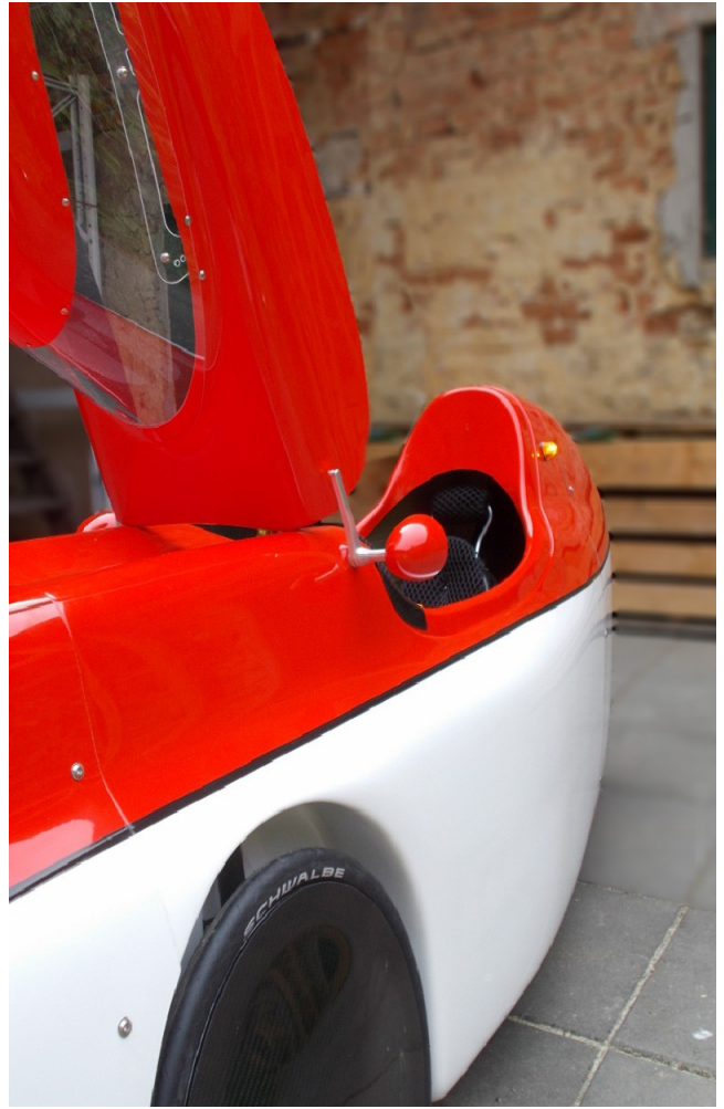
Race cap open for entrance and ventilation at stops/traffic lights etc. Visible carbon fiber wheel caps etc.
