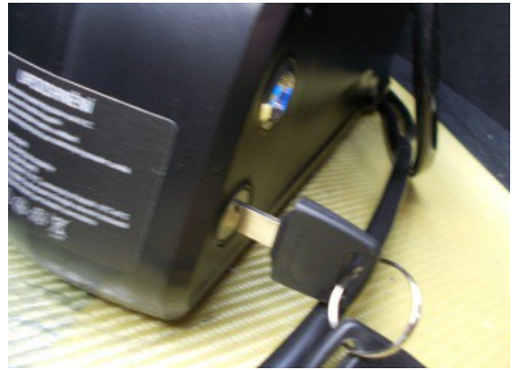
Lockable driving battery for E-WAW.
