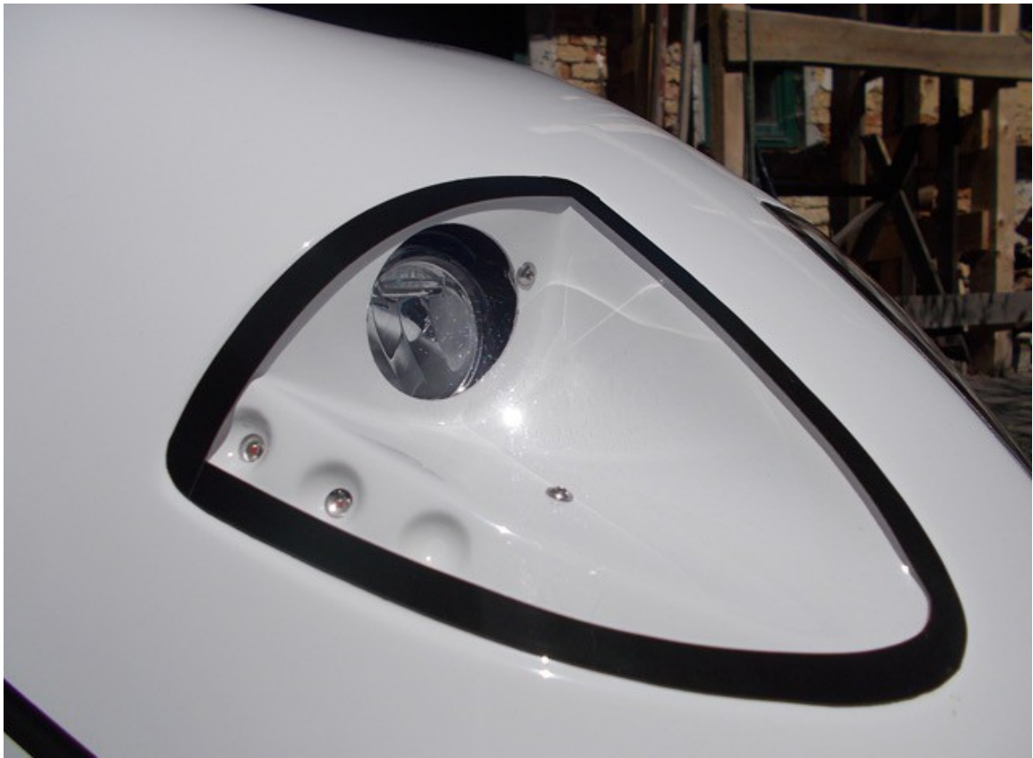
New integrated Bauch&Müller headlights, led blinkers.
