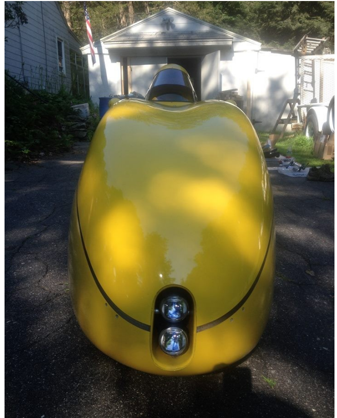
SPAI/Ventilation opening with 2 beam headlight LED blinkers and daylight integrated in the nose
