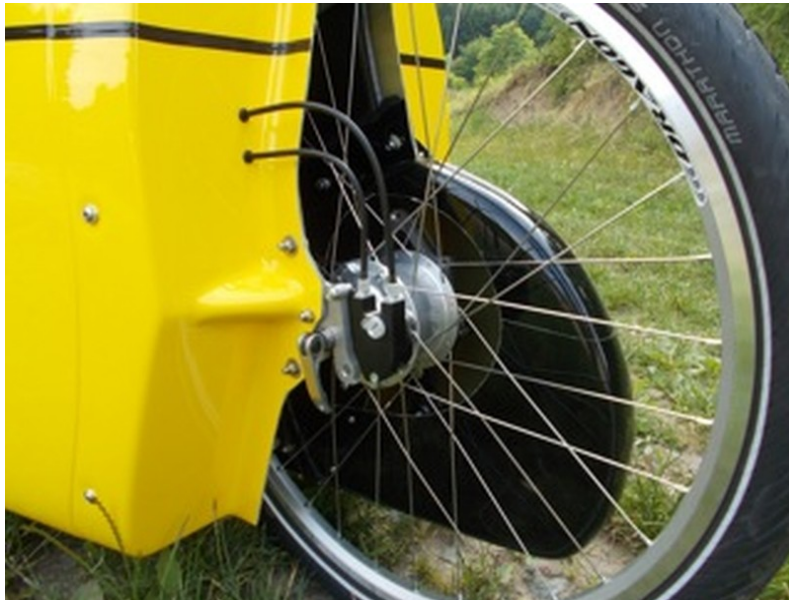
Rear chain and derailleurs protection (black). Recommended for winter/muddy conditions.
