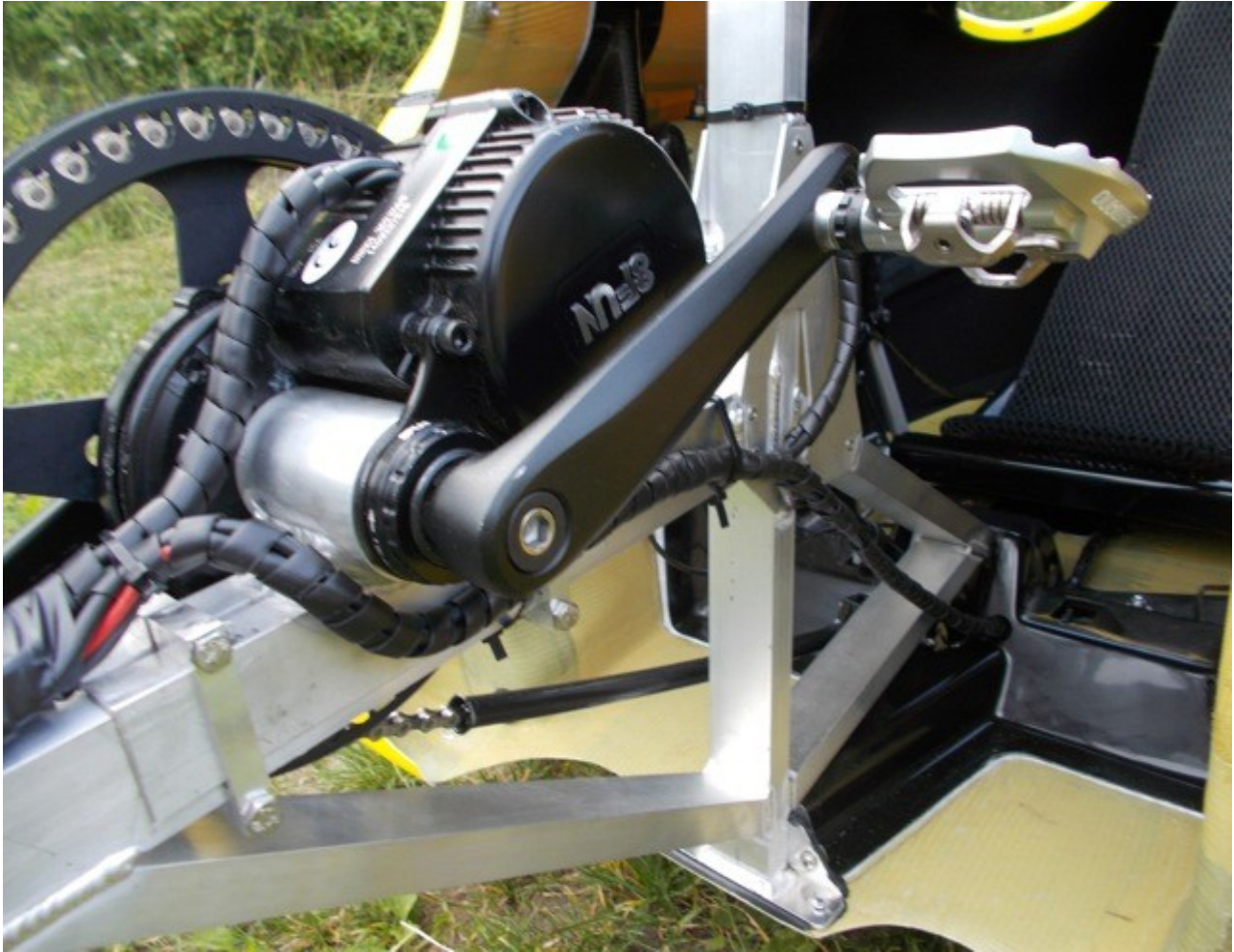
Bafang motor connected to front crank with free wheel, makes pedaling with or without motor assist possible. Programable speed limiter according to local restrictions. Delivered with 25 km/h setup (EU standard).
