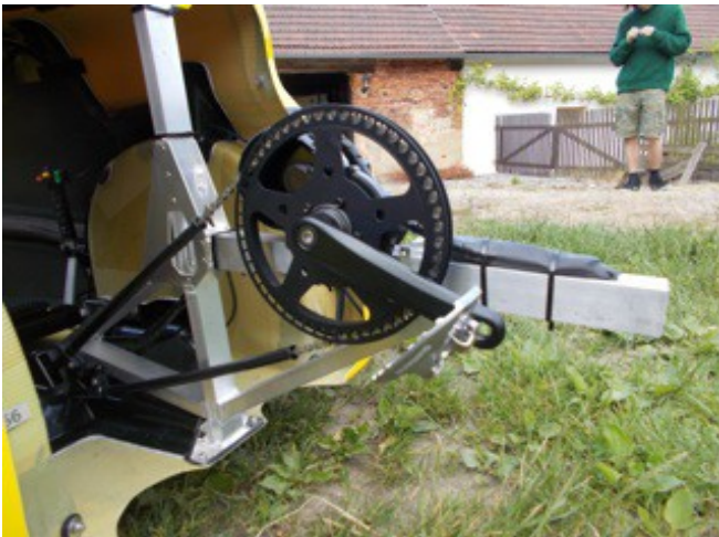
Front crank with 155mm crankarms
