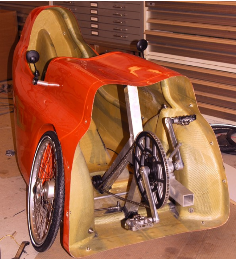
Mountain Drive with 65t (1:1), gears down to 26t (2,5:1). Gear shift with the heel, shift button in the crank.
