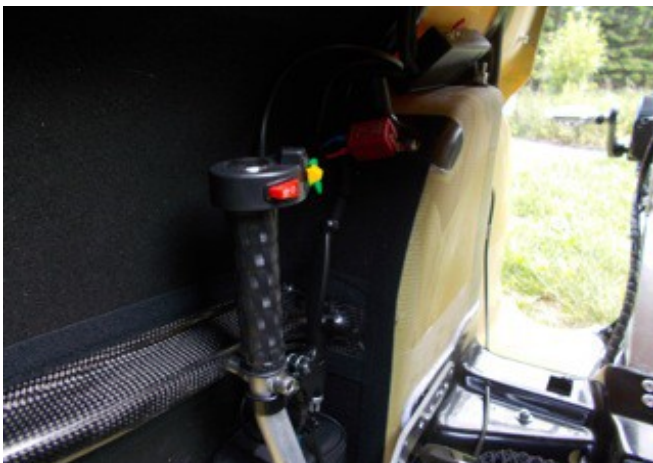
Left steering handle with light controls and horn. Placement of battery for E-WAW behind seat
