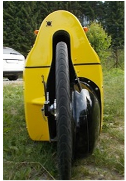
Rear chain and derailleurs protection (black). Recommended for winter/muddy conditions.
