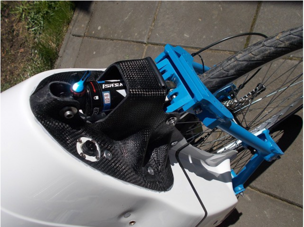
Connection and shock absorber mounted outside the body.
