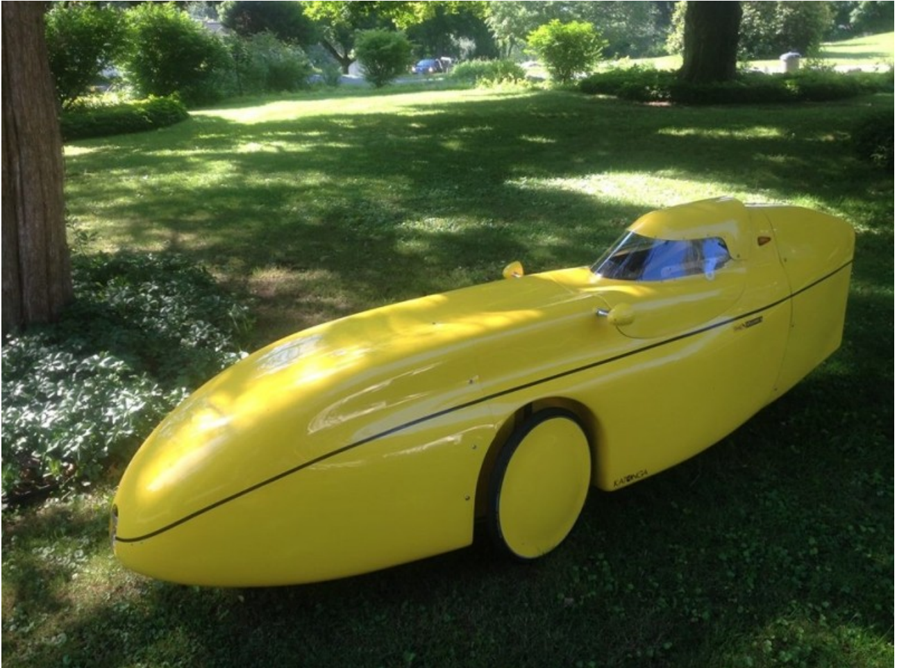
WAW256 with SPAI (ventilation in nose), wheel covers in carbon fiber, race hood, aerodynamic tail.
