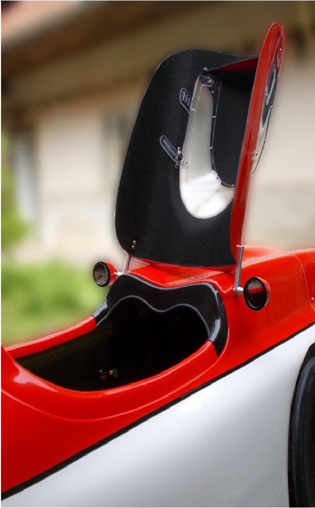
Race cap open for entrance and ventilation at stops/traffic lights etc. Visible carbon fiber wheel caps etc.
