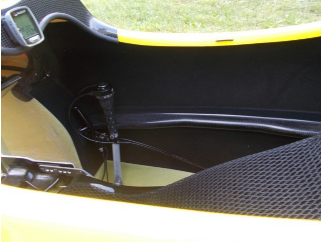
Detail of acoustic lining, hinged mesh seat(Ventisit), steering handle with brake and gear shifter http://rohloff.de Driving computer.
