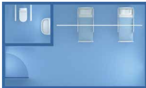
A straight track for two-bed coverage.
