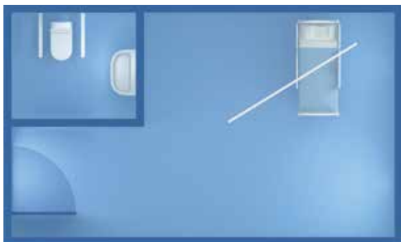
A straight track intended for transfers between bed and wheelchair.
