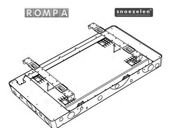
3. Hold the panel where you would like it to be mounted ensuring it is level. Whilst in position mark where the centre of the bracket mounting holes are on the wall. Do this for all 4x bracket mounting holes.
