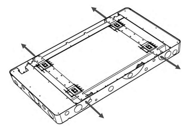
1. Unscrew the 4x M4 screws which secure the 2x brackets to the panels. The brackets are secured to avoid any damage during transit.
