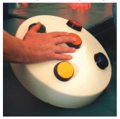
Switch off the Giant Maxi Bubble Tube completely. Connect the 5 Button Switch Box to the RJ45 socket in the base of the Giant Maxi Bubble Tube (the socket to the right of the SPEED dial). The protective cover will have to be removed first and stored in a safe place so it can be replaced after use.
