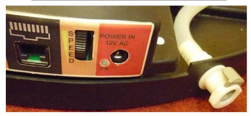
To remove the drainage tube, push on the grey button to release the tube. Removing the drainage tube automatically seals the cloudy pipe of the bubble tube. Empty any water that has remained in the drainage tube. Keep a piece of paper towel to hand to place under the white socket to catch the small amount of water that can be released.
