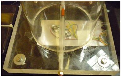
4. Attach the cloudy plastic pipe to the blue valve on the Bubble Tube column.
