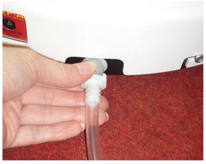
Connecting the drainage tube to the filling pump tube (to be purchased separately):
