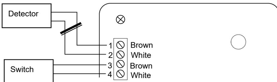
**NOTE:** If the external detector and the control switch is connected and programmed for the same terminal, any short circuit of the detector/detector cable will be registered as a press on the control switch, and the relay is activated (door opens!).
