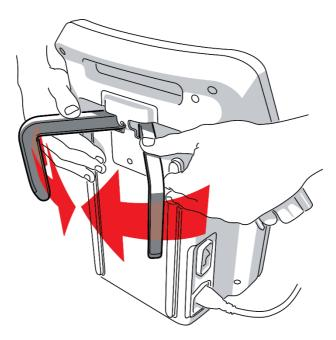
4. Hang the unit onto the bed frame at the foot end of the bed with the control panel facing outwards .
