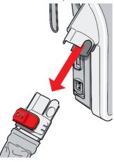
Simply push the buttons on the sides of the umbilical dock and the umbilical will disconnect. The mattress itself will remain inflated for several hours.
