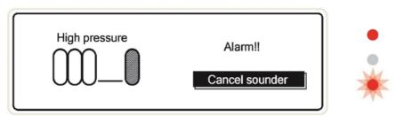
To resolve this issue, carefully push the CPR button and let out a small amount of air and then re attach the hose end. Reset the pump afterwards. Persistent high pressure alarms may indicate an internal fault. If if this occurs mattress system use should cease. The pump should immediately be sent for Servicing
