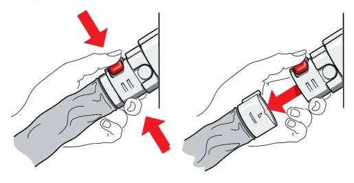
To deploy this emergency system, simply grip the CPR unit and push the RED BUTTON. The hose end closest to the mattress should spring out and the mattress will rapidly deflate.
