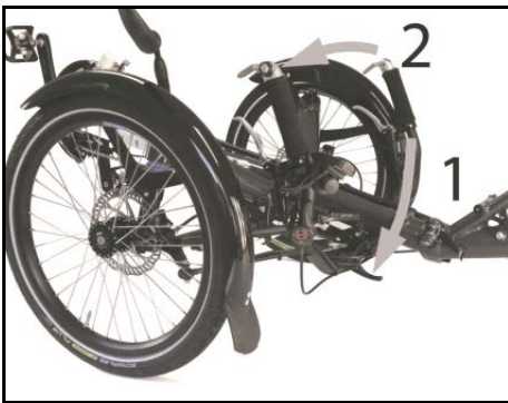
The handlebar on tricycle of the Scorpion series allows adjustment in width (1) and angle (2)
