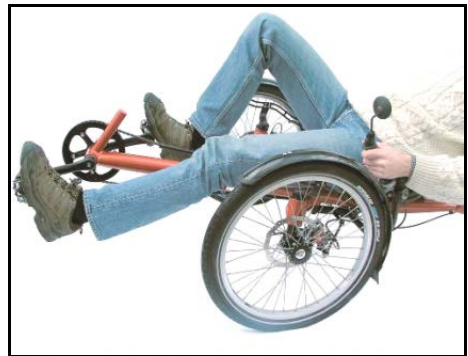
Adjust the front boom so that your knee will not be fully straightened when pedalling.
