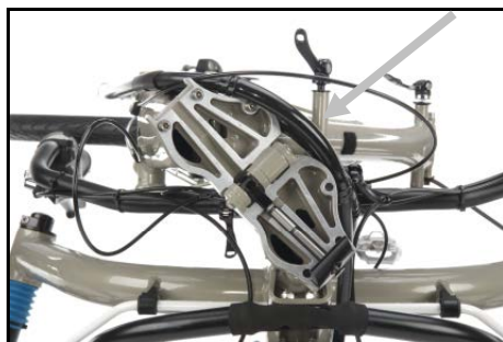
Move the chain tubes besides the folding hinge
