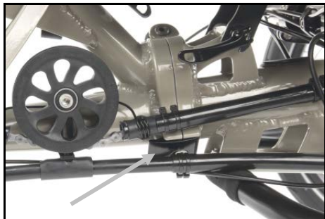
Securing tab on a Scorpion plus 26
