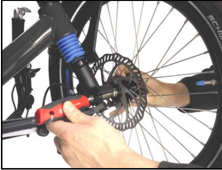
Loosen the screw in the locking part
