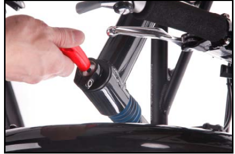
Loosen the hex head bolt on the clamp before adjusting the-pre load
