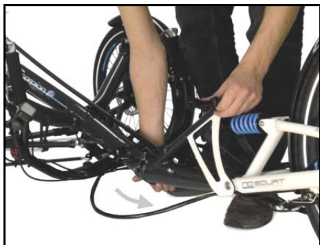
Opening the securing tab of the folding hinge
