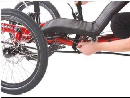
Handlebar width is adjusted at the stem clamp under the seat.
