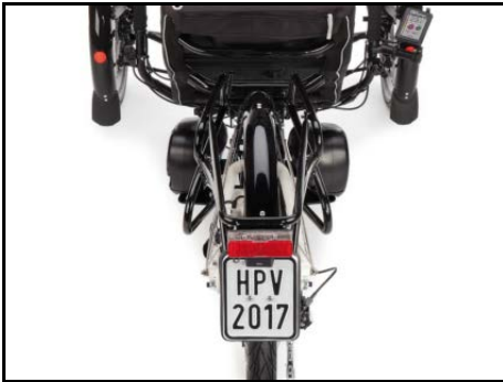
The S-Pedelec rear light features braking light and license plate illumination
