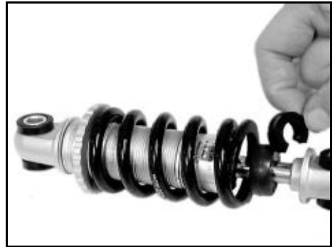
The suspension travel is adjusted by adding clips to the piston rod of the spring element.
