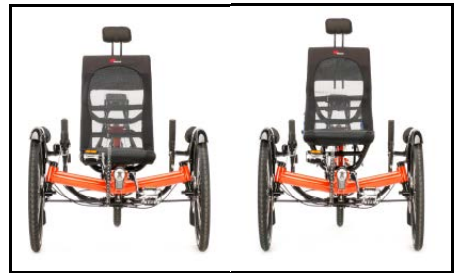
ErgoMesh-seat standard (l.) and ErgoMesh HS (r.)
