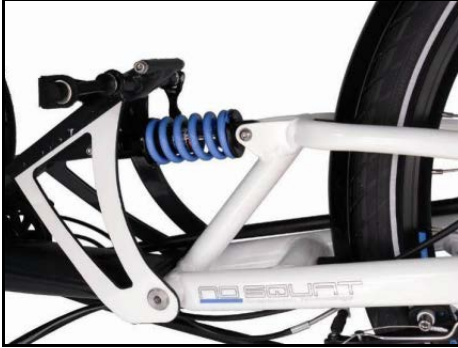
Steel spring suspension element with fixed damping rate.
