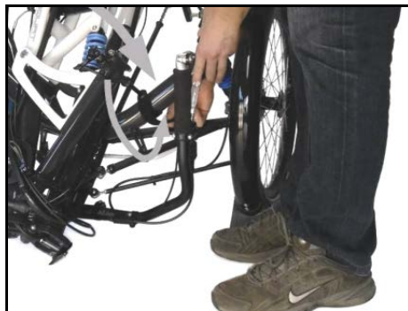
Locking the frame with the hook-and-loop strap on the cross tube
