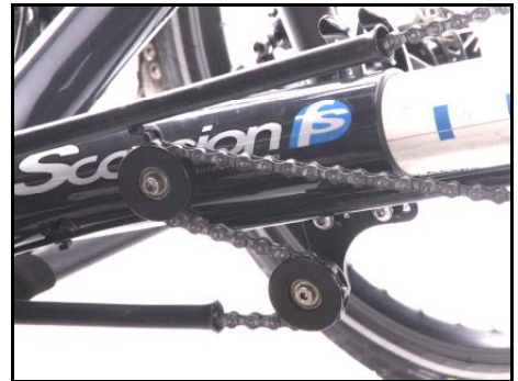
Routing of the chain over the idlers of the front boom quick adjust
