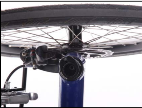
View into headset with star flanged nut inside
