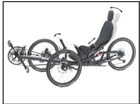
Seat adjustment on tricycles with BodyLink-seats
