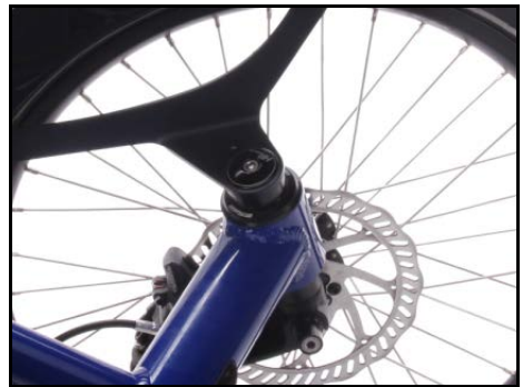
The holding sheet of the mudguard is fixed with the cap to the headset
