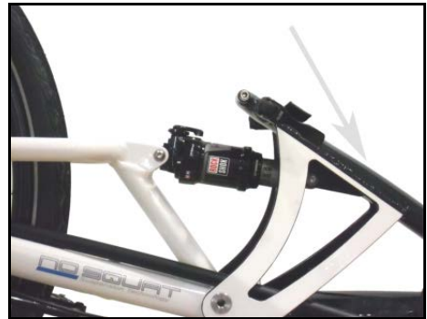
Position for identification mark on the Scorpion fs 26 frames
