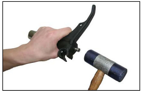
A hammer punch on the bolt releases the piston inside the knuckle.
