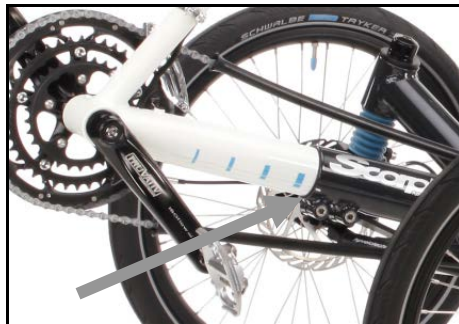
Mark on the front boom of the Scorpion fs 26
