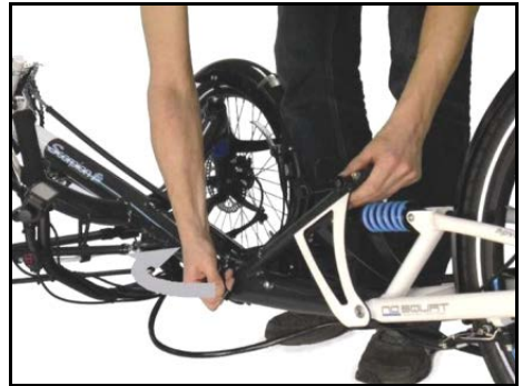
Opening the quick-release lever of the folding hinge
