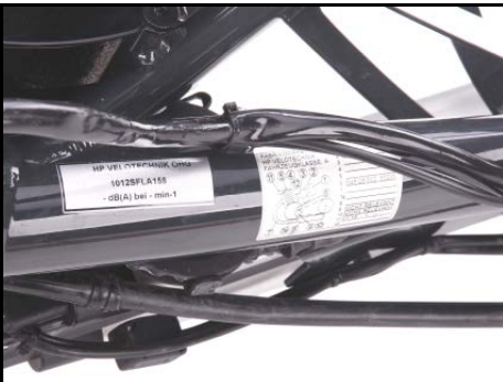
Identification- and anti-manipulation plate
