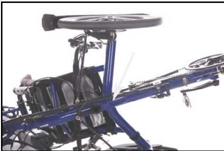
Position of frame number on Gekko models
