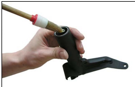
Applying grease to the bushings.
