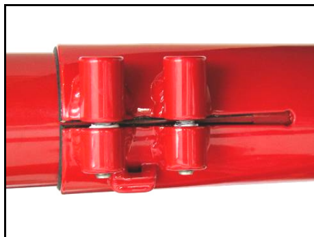
The rear end of the front boom must never be visible in the clamping slot.
