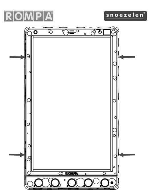
4. Secure both brackets to the wall\* ensuring the centre of the bracket mounting holes line up with the marks just made to ensure the bracket it level when mounting it to the wall. The top bracket mounting holes should line up with the top 2x marks and the bottom bracket mounting holes should line up with the bottom 2x marks.
