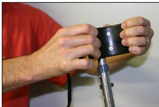
Figure 3: Keeping of the desired shape during cooling of the plastic part
